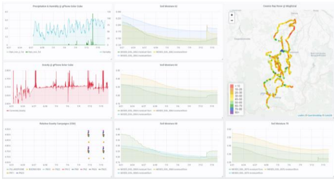
Figure 7: Demonstrator of the Observatory View with data from the MOSES Müglitztal Campaign 2019. Gravimetric data for near-surface water balancing (GFZ), in-situ mobile wireless sensor network (UFZ) and mobile Cosmic Ray Neutron Sensing (CNRS, UFZ) data for determination of the soil moisture are shown.
